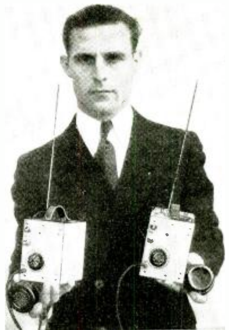
The author with two of his "Transceiver" units. Each is complete with self-contained batteries. Flip a switch to talk or receive.
