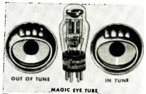
MAGIC EYE TUBE The appearance of the "Magic Eye" when the tuning is off resonance (left) and when on the exact resonance point of the station (right).
