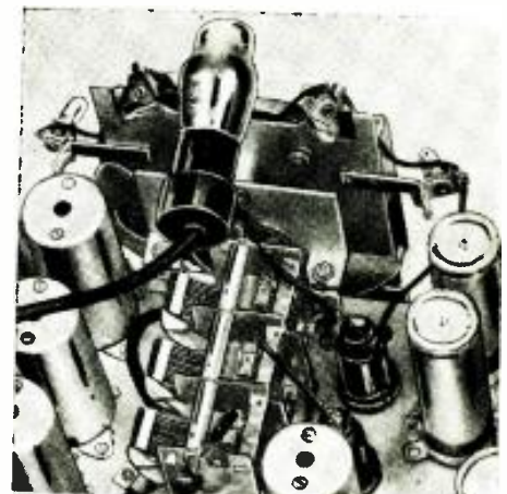
The "Magic Eye" tube, type 6E5, is mounted just above the tuning dial on the front of the chassis as here shown.
